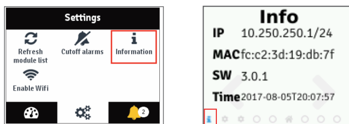
Figure 3: Inview S and Inview S Slot - LCD display - Info page
